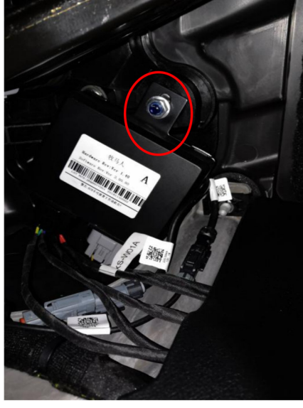
9) Fix the ECU with M8 Screw
