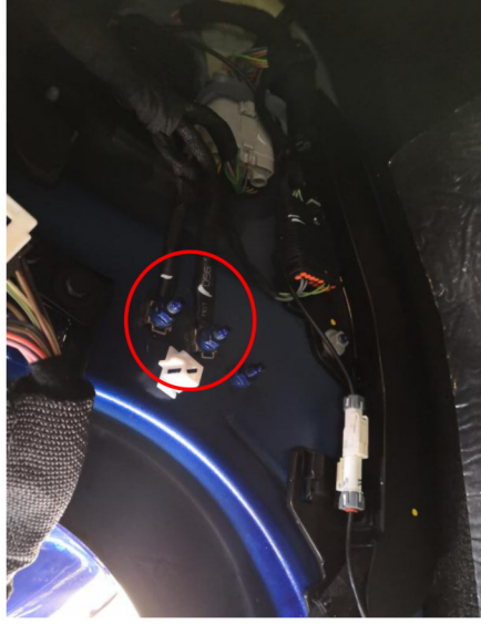
7) Connect negative pole to this place
