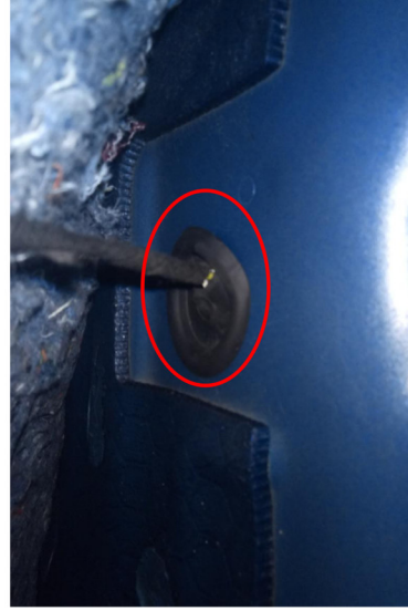
10) Link one motor line from the carpet to the chassis
