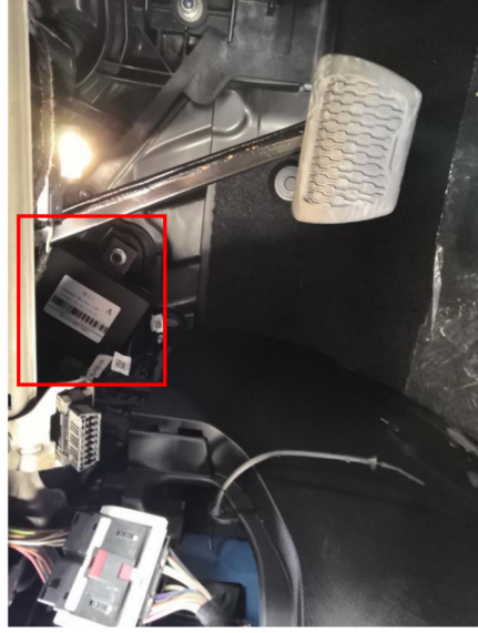
8) Fix the ECU in the driver room
