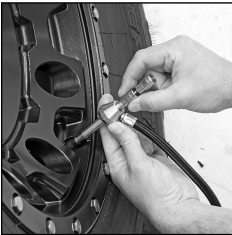
10) Hold the sliding valve and unscrew the valve stem adapter from your valve stem.
