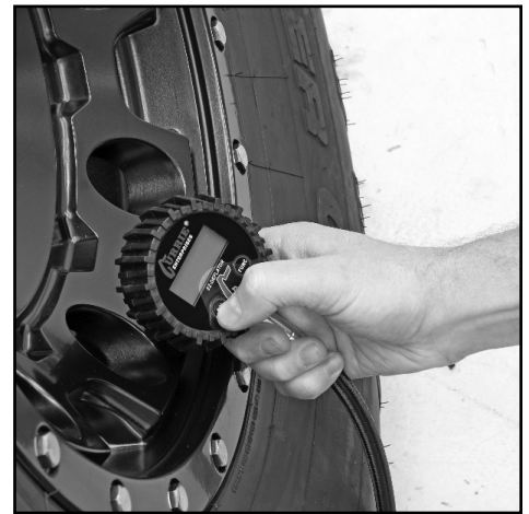
12) Click the "ON" button once to power the unit off. Unit will power off automatically after 2 1/2 minutes.
