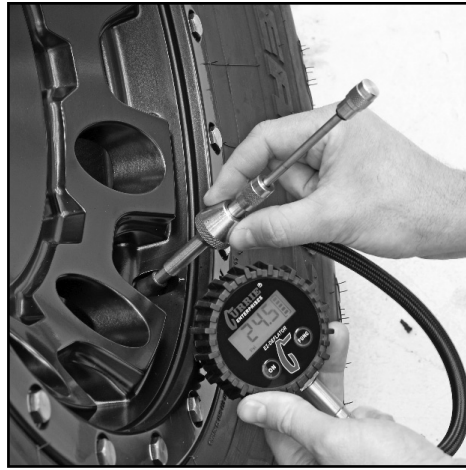
8) Push the sliding valve back down to check the new tire pressure. This tire is now at 24.5 pounds.
