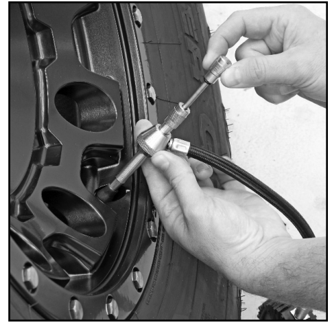
9) Once you have reached your desired tire pressure, screw your valve stem back in using the valve core remover.
