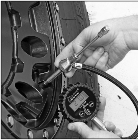
7) Pull the sliding valve up to start releasing air from the tire. Air will flow rapidly! Disregard the gauge reading during that the time the sliding valve is pulled out.
