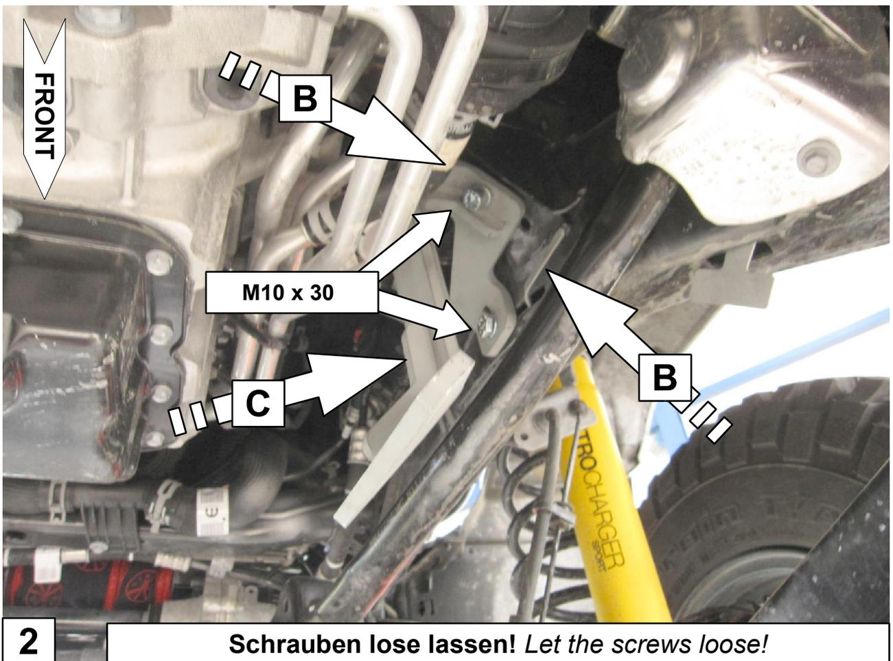
Schrauben lose lassen! *Let the screws loose!*
