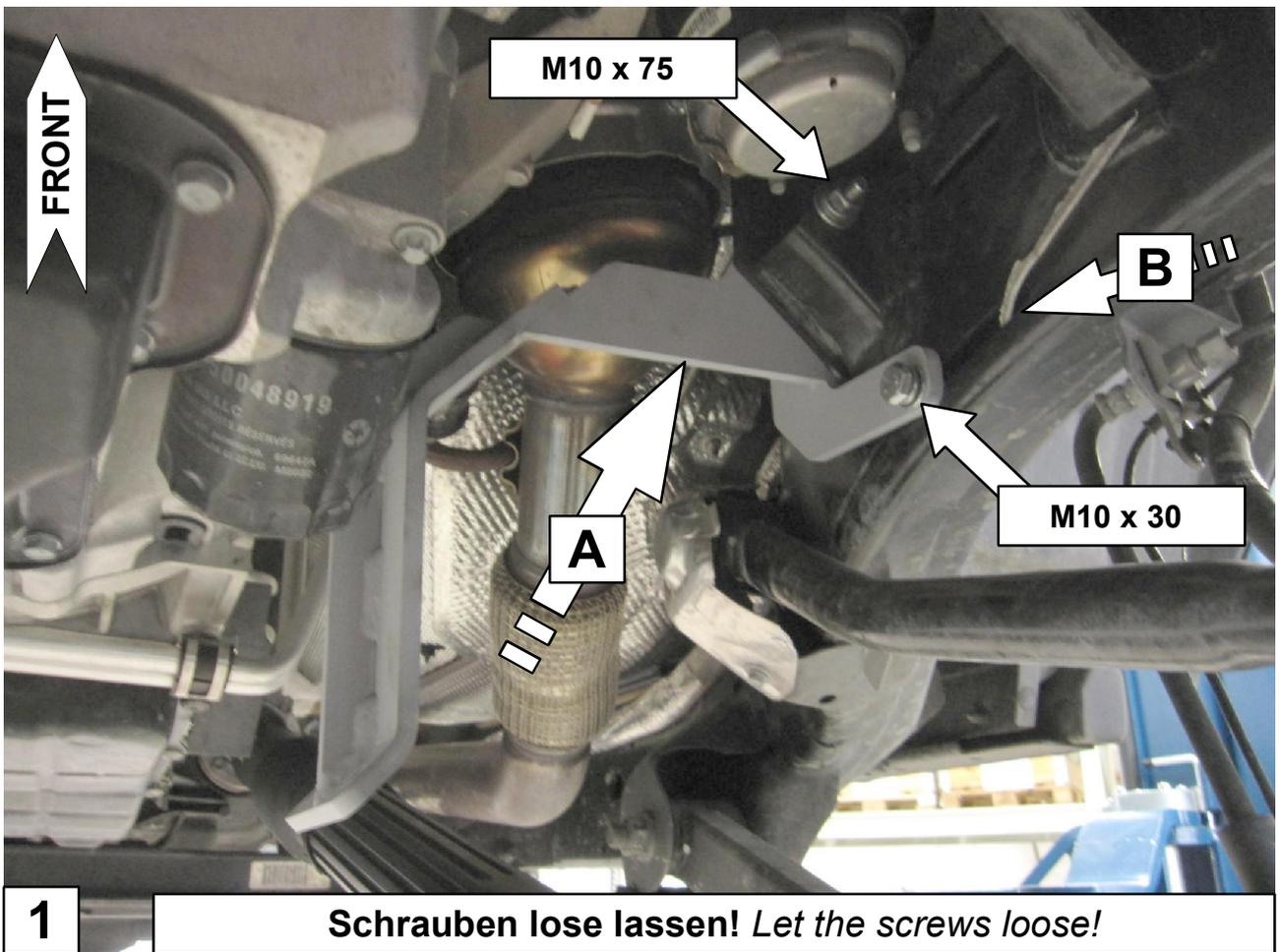
Schrauben lose lassen! *Let the screws loose!*
